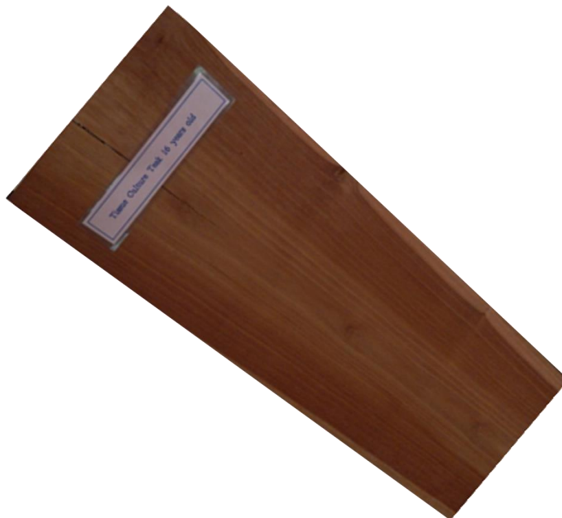
Flat-sawn board from 16 year old Tissue cultured teak (Note the uniform wood colour)
